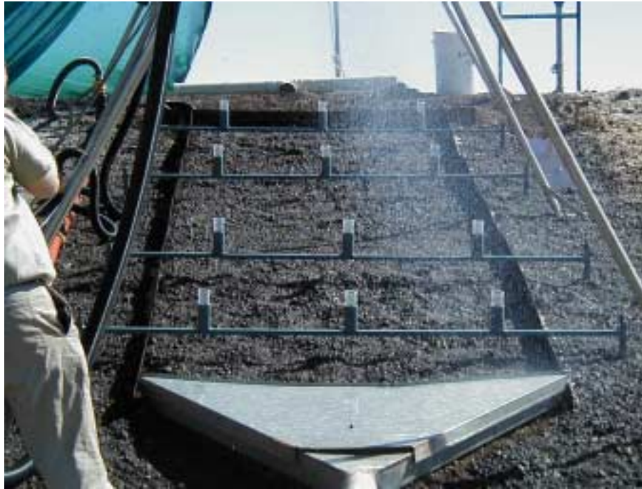
Figure 3: Rainfall simulator plot (control treatment), showing rain gauges, plot boundaries, and installation for collecting runoff.
