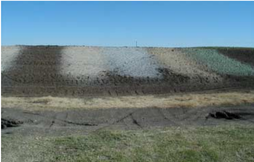
Figure 1: View of study area prior to testing, with different hydromulch materials applied
